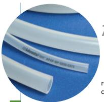
dvantaFlex TPE (thermoplastic elastomer) tubing addresses the need for a flexible, translucent, sterilizable, moldable, heat sealable, and weldable biopharmaceutical tubing for fluid processing. AdvantaFlex maintains its physical properties following sterilization processes, resists kinking, remains translucent for visible product flow, and does not become gummy.
